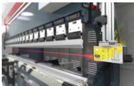
CE Laser Safety System
